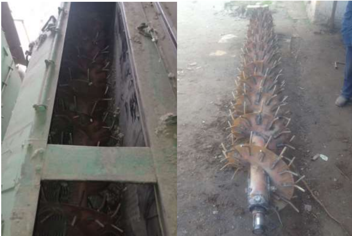
Figure 2. General view of the improved screw conveyor installed on the 6A-12M equipment.
